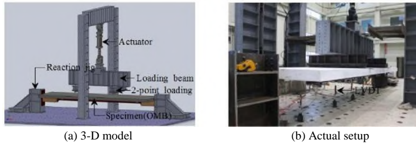
Fig. 4 Test setup for a typical specimen
