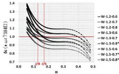
Fig.2 Variation in central deflection under uniformly distributed loads  $\omega$
