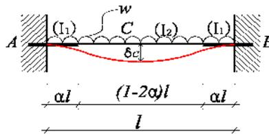
Fig. 1 OMB subjected to uniformly distributed load  $w$
