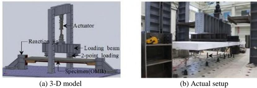
**Fig. 4** Test setup for a typical specimen
