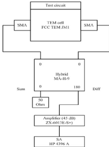
Fig. 1. Diagram of the test bench.
