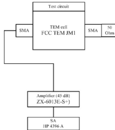
Fig. 2. BISS method to measure the radiated emission.
