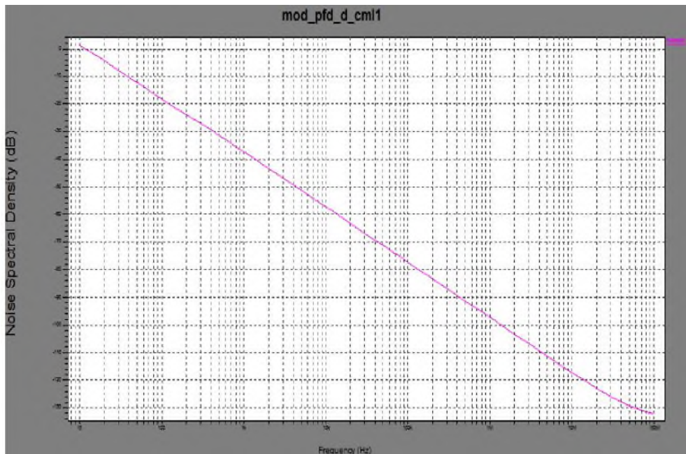
Figure 12. Noise Spectral Density Graph for M_CML_PFD (x Axis Represents a Frequency Range from 10 to 100 MHz and y Axis Represents Noise in db)
