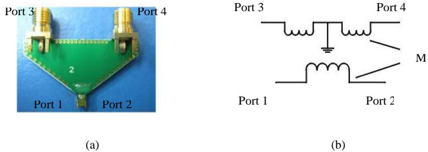
Fig. 2. (a) Current probe and (b) Equivalent circuit of the probe.
