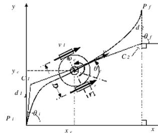
Fig. 1. Kinematics of TMR and Bezier Curve-based path planning
