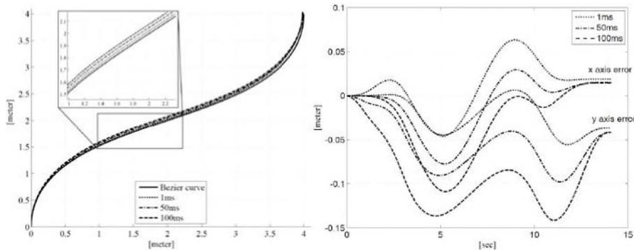
(a) Trajectories driven by central velocities      (b) Tacking errors along the Bezier curve
