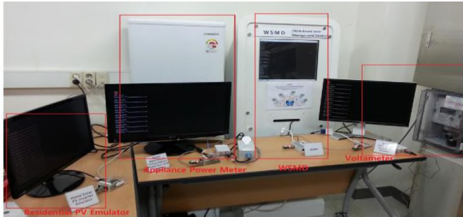
Fig. 3. Demonstration Setup (left: Residential PV Emulator, Appliance Power Meter, Web-based solar monitoring device, and Voltmeter)
