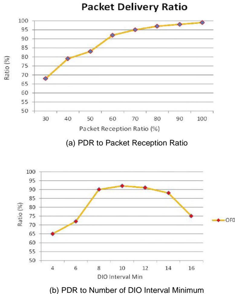
**Figure 13. Packet Delivery Ratio (PDR) of Objective Function**
