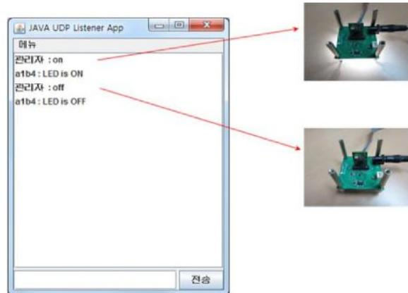
**Figure 10. LED Sensor Control Program and The**
