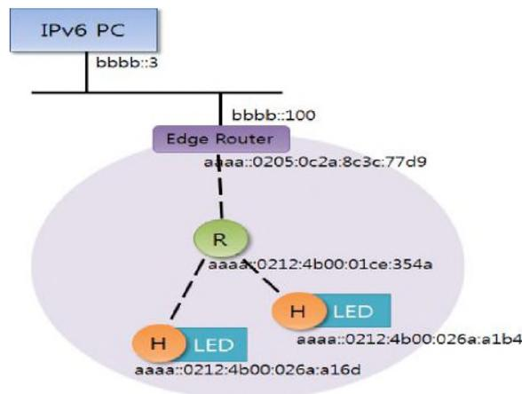
Figure 8. Simple IPv6-USN
