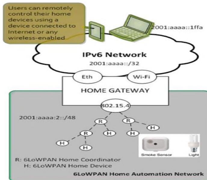
**Figure 1. IPv6-USN Home Automation System Architecture**
