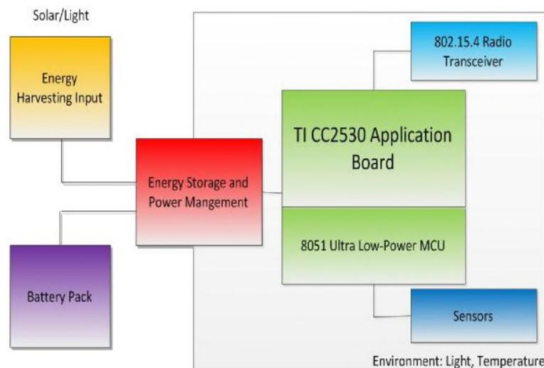
**Figure 4. IPv6-USN Home Automation Nodes with Energy Harvesting**
