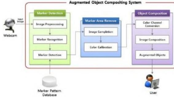
Fig. 1. Diagram of design of augmented object compositing system based on diminished reality
