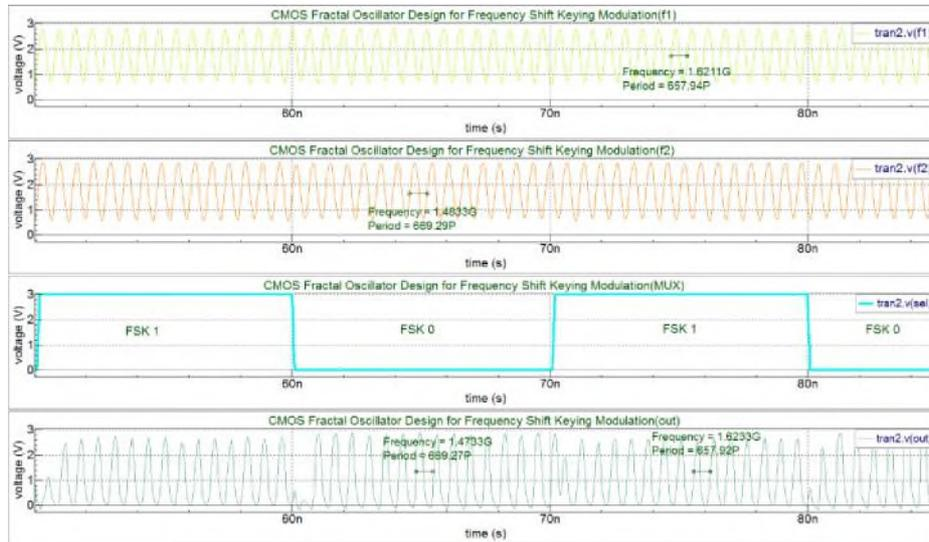
**Fig. 5.** SPICE simulation results for the FSK modulation: (top to bottom) f1, f2, SEL, and FSK modulation
