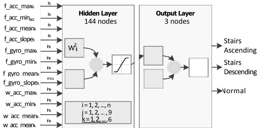
Fig. 2: Neural network architecture for step terrain characterization
