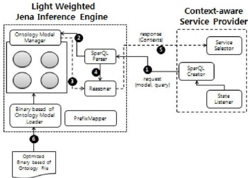
Fig. 8. Light weighted Reasoning Engine and Context-aware Provider Structure
