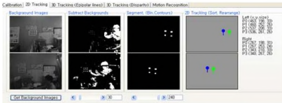
Figure 3. Preprocessing and acquiring 2d data points
