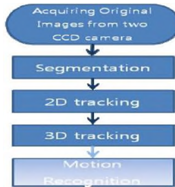
Figure 1. Operating procedure of the motion capture system
