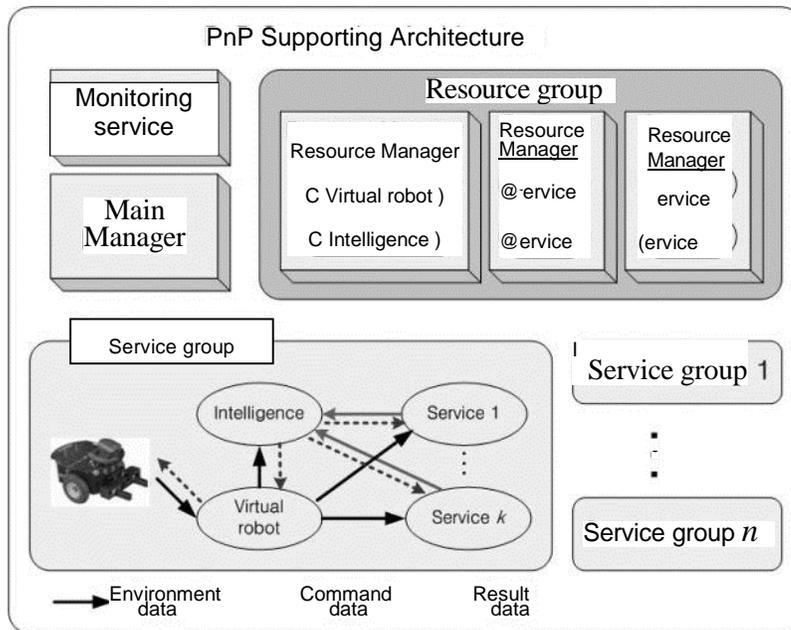
**Fig. 1.** The configuration of PnP architecture.
