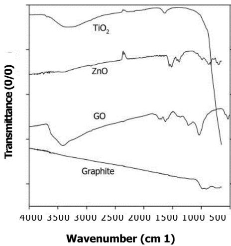
Fig. 1. FTIR spectra of photocatalysts used.
