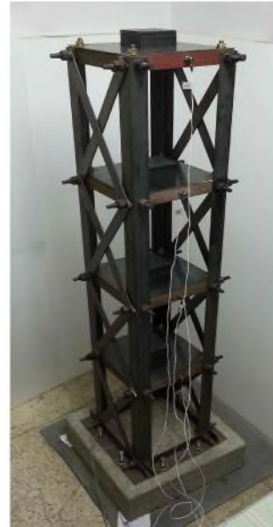
Fig. 2. Steel frame model structure
