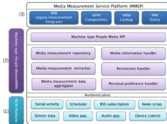
Fig. 2. Architecture of Machine-type Media Measurement System
