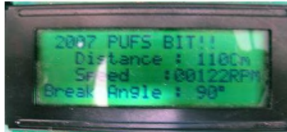
Figure 8. LCD screen displayed distance, speed, and angle
