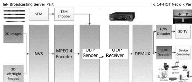
Fig. 2. System concepts of 4D real-sense media broadcasting service system.
