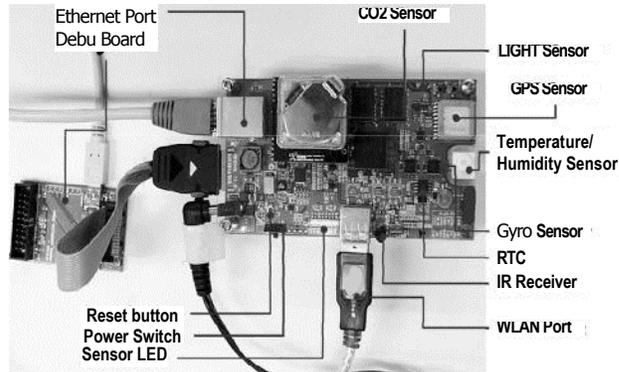
Fig. 5. Implemented aggregator with multiple real-sense sensors.
