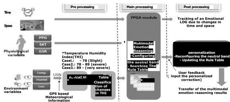
Fig. 2. Architecture of the multimodal emotion reasoning engine
