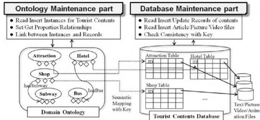
**Figure 8. Diagram of Roles and Relations among Ontology Maintenance and Database Maintenance Parts of the TCS System**
