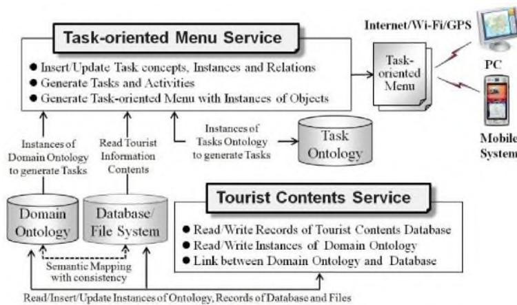
**Figure 7. ITISTO System Architecture with Ontologies and Database**
