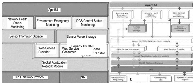
Fig. 3. Architecture of AMS (a)Block Diagram, (b) Function Flow
