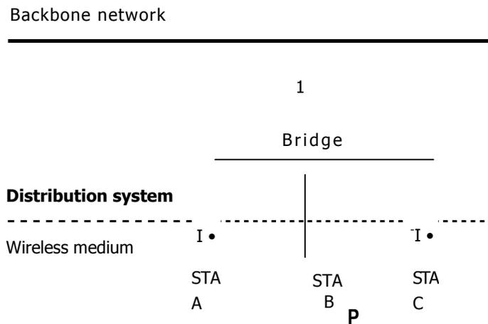
Fig. 1. The distribution system in IEEE 802.11
