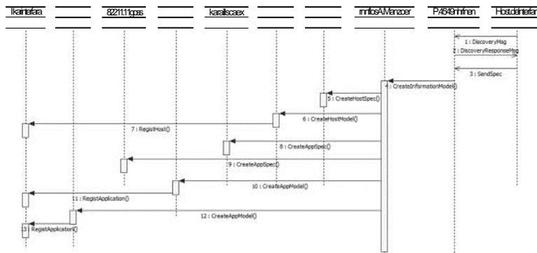
Fig. 3. Sequence Diagram for Constructing Information Model
