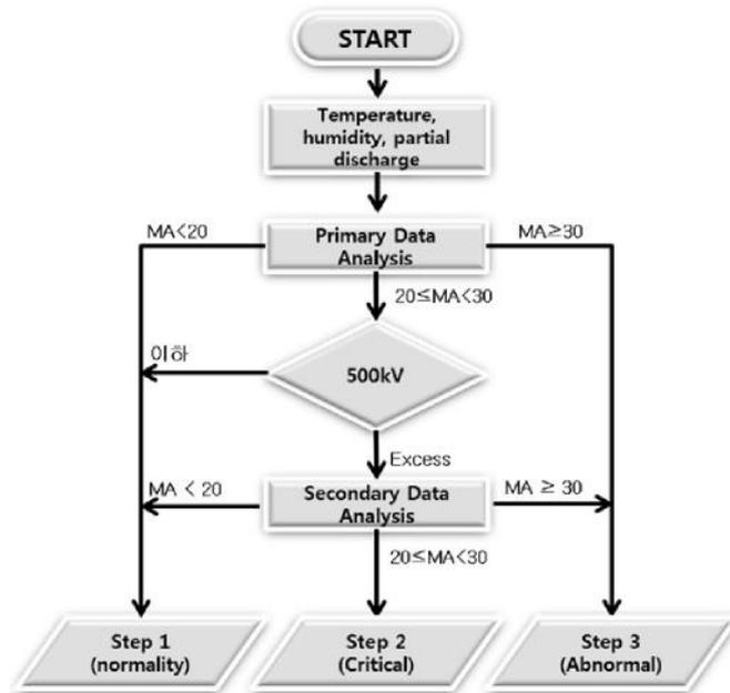
Fig.3. Deterioration calculated by checking the state of aging
