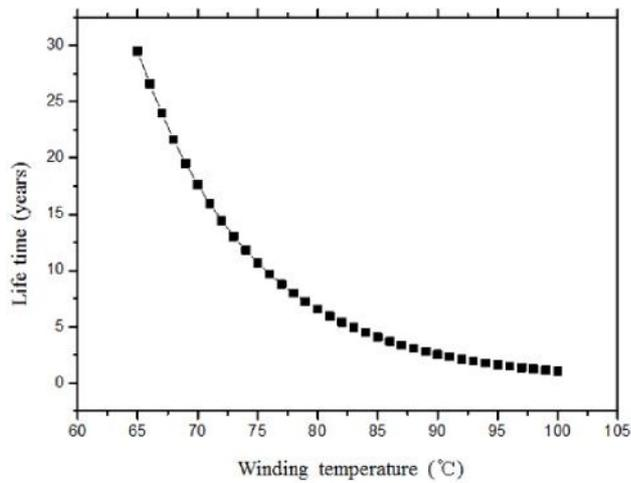
Fig.2 Life prediction of Mold transformer using the Arrhenius equation
