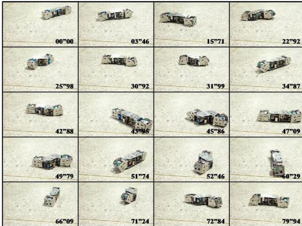
**Figure 13. Combined Motions including Snake Motion**
