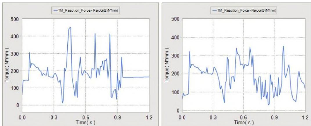
**Figure 7. Torques of 2<sup>nd</sup> and 3<sup>rd</sup> Module at Inchworm Motion**
