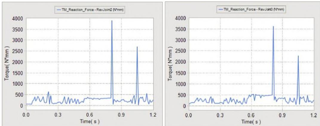
**Figure 9. Torques of 2<sup>nd</sup> and 3<sup>rd</sup> Module at Butterfly Motion**
