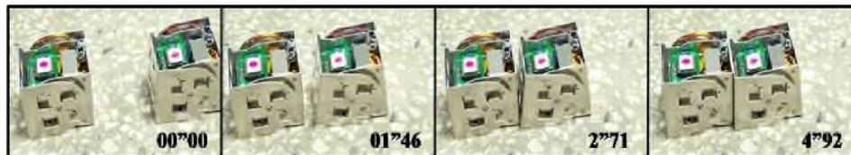
**Figure 12. Moving Independently, Docking, and Inchworm Motion**
