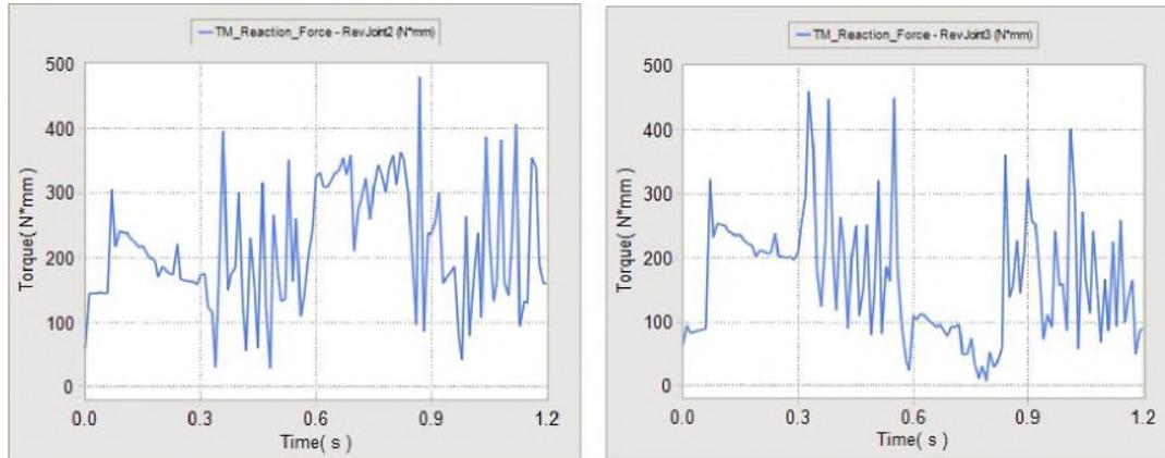
**Figure 11. Torques of 2<sup>nd</sup> and 3<sup>rd</sup> Module at Snake Motion**
