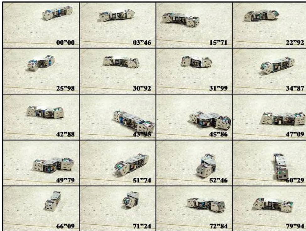
Figure 13. Combined Motions including Snake Motion
