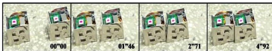
Figure 12. Moving Independently, Docking, and Inchworm Motion
