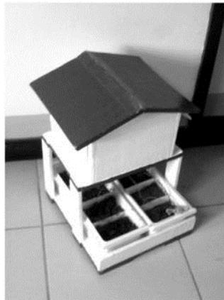
**Fig. 4.** This figure shows a prototype of the powerhouse that should be sited in a remote area where the sensors are attached. It provides a voltage and current supply for the remote sensors
