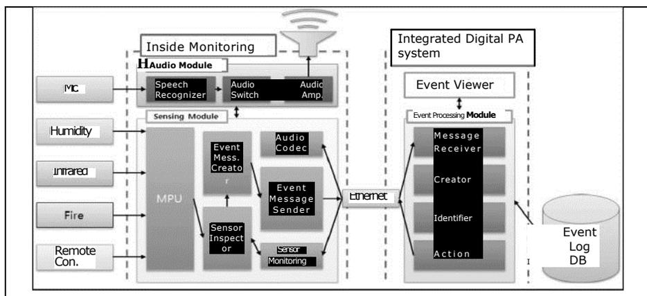
Fig. 1. System structure
