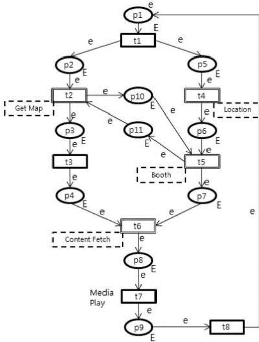
**Fig. 1.** A hierarchical Petri net model of a location based VOD client system
