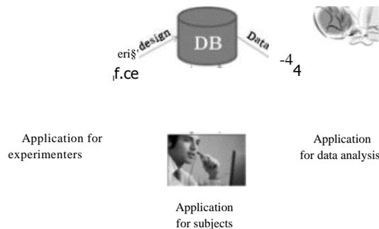
(Fig. 2) Three applications forming the IVR system simulator
