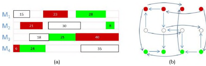
Fig. 1 A possible schedule for an OSS with 3 jobs and 4 machines is given by (a) a machine-oriented Gantt chart, and (b) a sequence graph.
