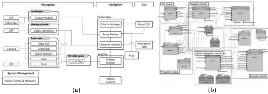
**Fig. 2.** (a) Autonomous vehicle system architecture, (b) OPRoS components and their connections
