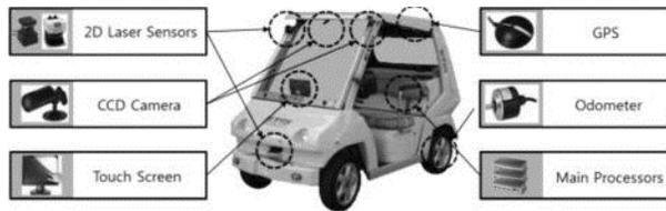
Fig. 5. Hardware configuration for ESTRO.
