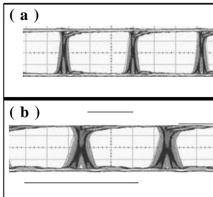
Fig. 3. Eye-diagram for (a) 622Mbps and (b) 1.25Gbps.
