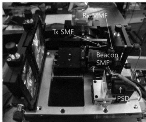
Fig. 2. Photograph of the assembled TRM.
