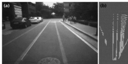
**Fig. 6.** (a) Detected lane with the Hough transform overlaid onto the original image (b) Local map 2D Boolean array
