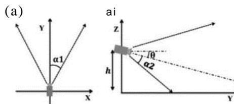
Fig. 3. Geometrical parameters for the Inverse perspective transform
