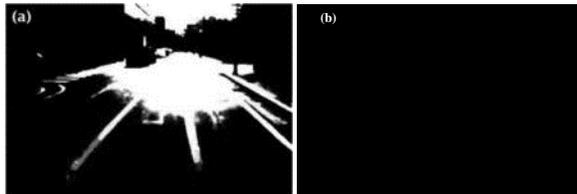
Fig. 2. (a) A road image showing light spreading phenomenon with contrast image processing (b) A processed image showing the difference between background and original image after fixing light spreading phenomenon.
