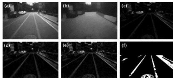
**Fig. 5.** (a) Original image (b) Background image processed with the morphological operators ("Erode" and "Dilate") (c) Image with the background eliminated (d) Image with the Median filter used (e) Image with the Highlight convolution (f) Binarized image with the ROI extracted.
