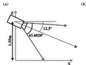
Fig. 1. (a) Camera setup parameters (b) 2D Boolean array with 3200 bits (80(V)x40(H)) in the ROI.
