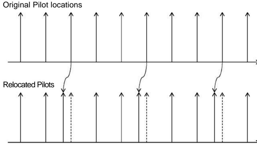
Fig. 2. The conceptual illustration of pilot relocation method
