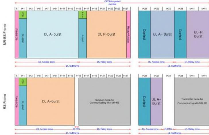
**Fig. 1.** Example of the TDD frame structure
