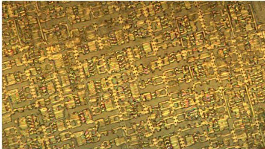
**Fig. 2.** The detail of an RFID tag – bare transistors can be recognised. This image was acquired by optical microscope Olympus BX61 with insufficient magnification abilities; our intention is to use an electron microscope to obtain better quality images for analysis.
