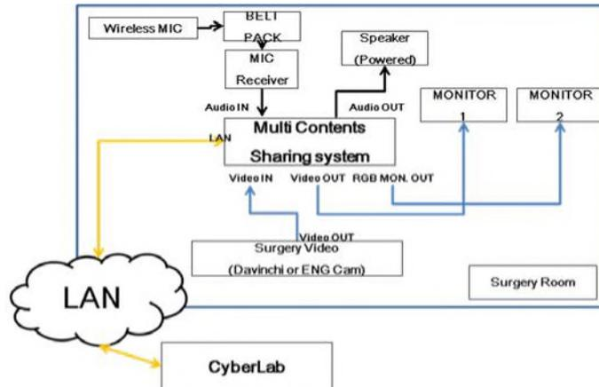
Fig. 3. Block Diagram for Bi-Path Live Surgery
