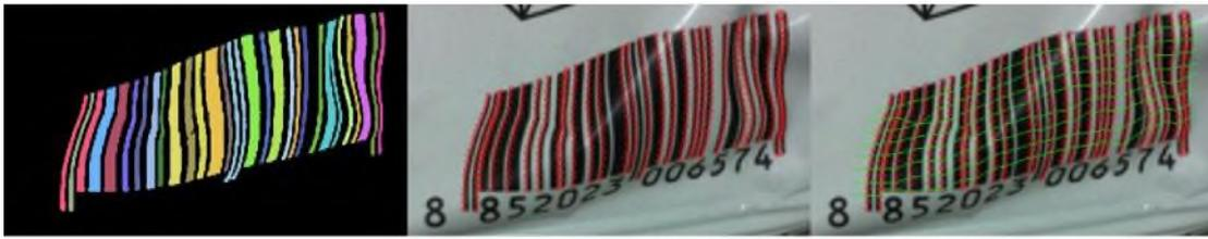
**Figure 5. Demonstration of Scanning Track Tracing. Anchor Points are Created on the Barcode Structure (middle), and Used to Generate Scanning Tracks (right)**
