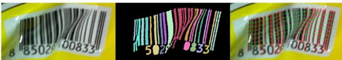
**Figure 10. High Degree of Bars Merging in the Middle Part of the Barcode Causes the Algorithm to Miss Some Elements**
