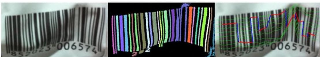
**Figure 11. Binarization Error Caused by Shadow Regions Makes the Algorithm Skip a Bar Element and Produce an Incorrect Decoding Result**
