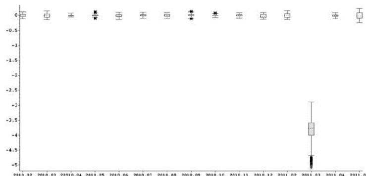
**Fig. 2.** Time-series of box plots with respect to the differences between multiscale geoid heights for the period from February 2010 to May 2011 and the multiscale geoid height for January 2010 selected as the reference. (unit: meter)
