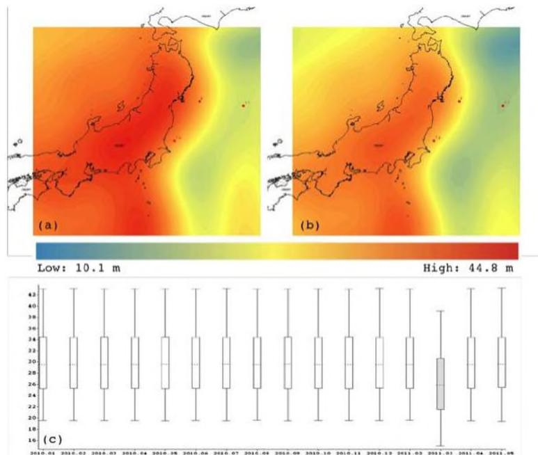
**Fig. 1.** Multiscale geoid heights using the Abel-Poisson scale function and wavelets on individual points of a  $0.1^\circ \times 0.2^\circ$ , (a) with range 19.467~43.054 m for February 2011 and (b) with range 14.890~39.789 m for March 2011. (c) Time-series of box plots with respect to multiscale geoid heights for the period from January 2010 to May 2011 (unit: meter).
