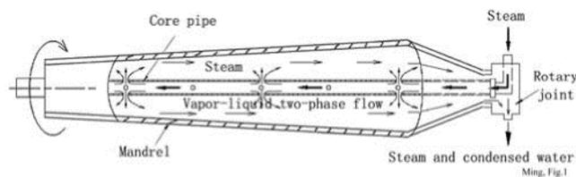
Fig. 1. The mandrel structure of the winding machine
