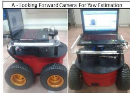
A - Looking-Forward Camera for Yaw Estimation
