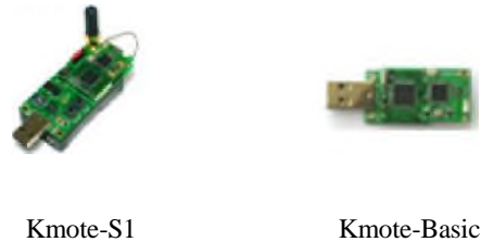
(Fig. 3 Sensor node and synch-node)
